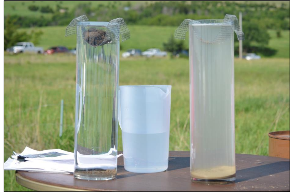
Slake Test: After 25 minutes. Water-stable structure on left. No structure on right. Consider impact on water infiltration, runoff, erosion, and surface water quality.
