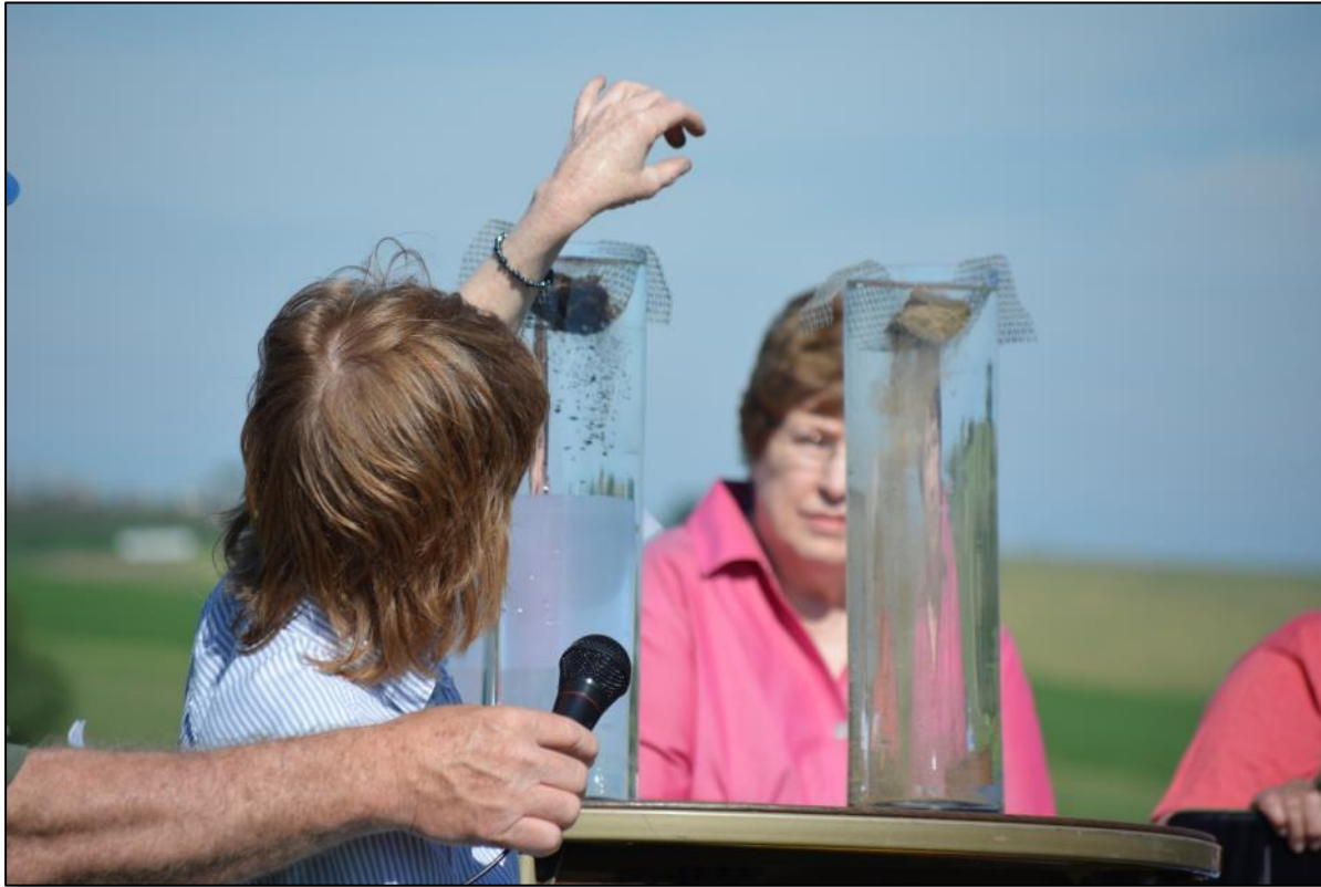
Slake Test: Peds from long-term grassland (left) and conventional tillage fields (right) suspended in water column.
